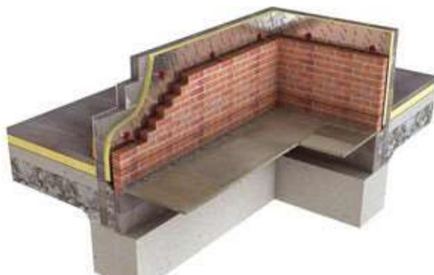
Standard UK brick/PU/block build
